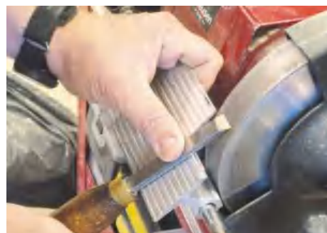
▲ Pic.3 If you need to sharpen on a platform, then try to get your hands in a position that allows you to slide the tool sideways
